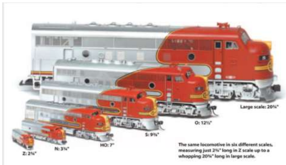
Figure 11- Comparison of Scale Sizes (Guide to Model Railroading Scales and Gauges | World's Greatest Hobby, 2016)
